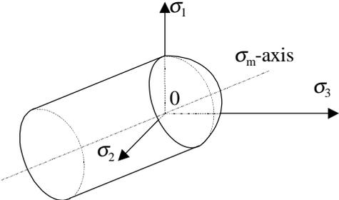
**Figure 2: Plastic potential for soil element**
