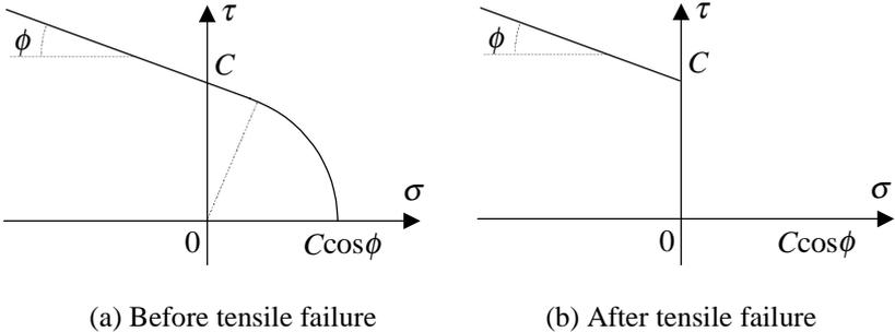
**Figure 1: Failure criteria for soil element**
