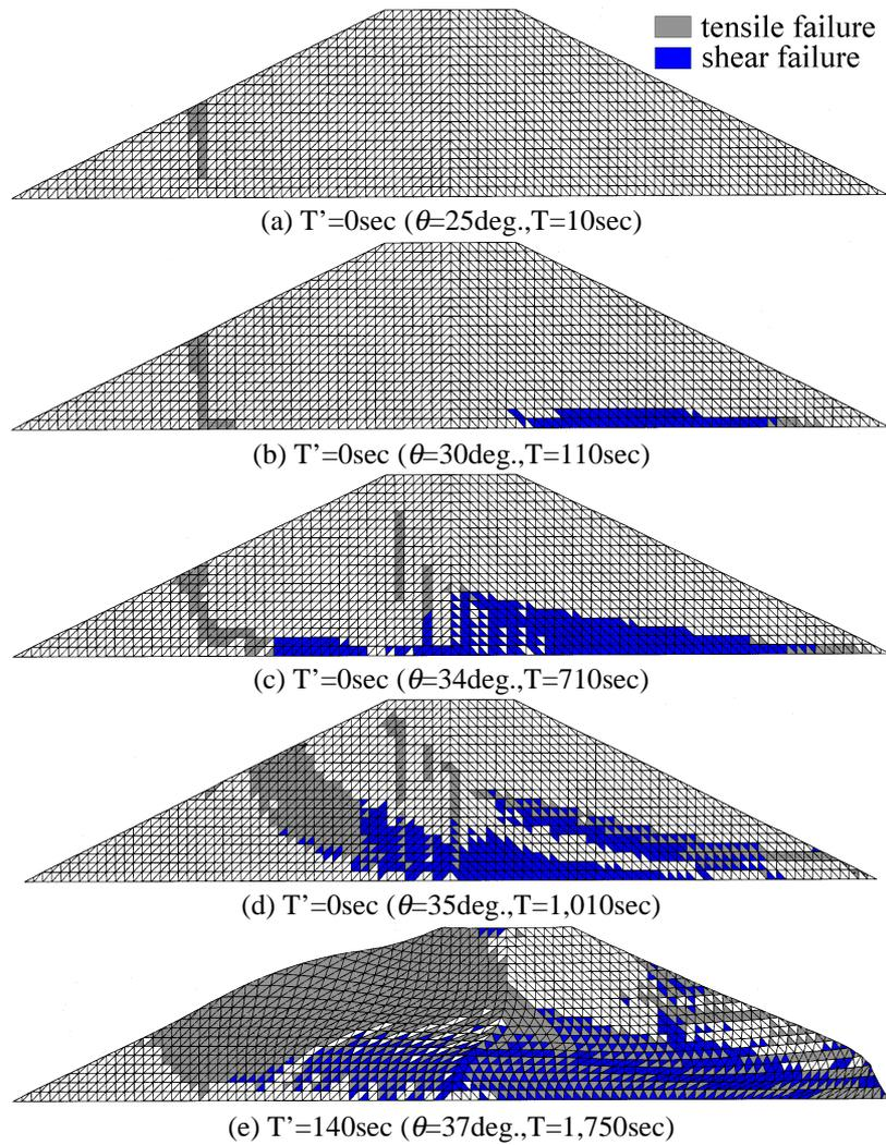
Figure 10: Collapsing process of the embankment
