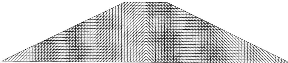
Figure 7: FE mesh to simulate the inclination test
