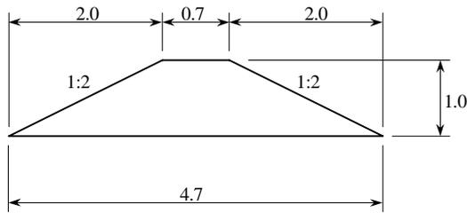
Figure 4: Embankment model for inclination test
