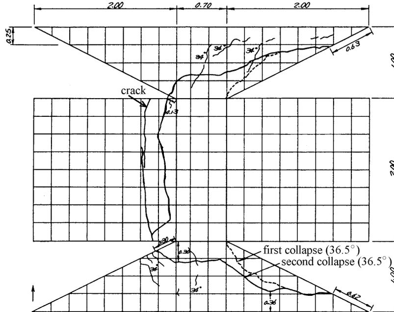
Figure 6: Distribution of cracks [Ito et al. 1982A]
