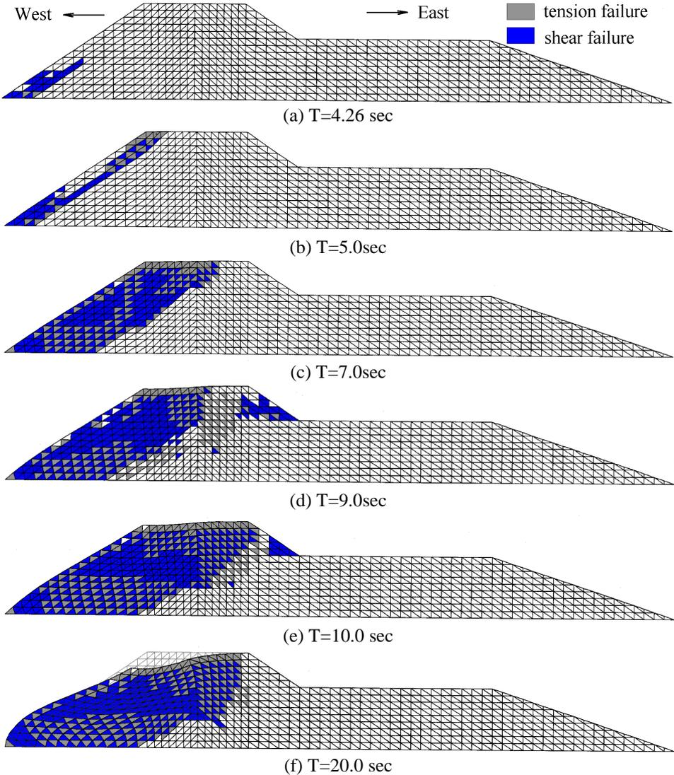
**Figure 15: Collapsing process of the embankment**
