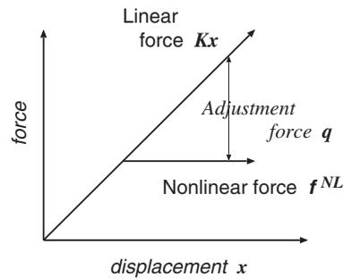
Figure 6. Adjustment force to consider the non-linear restoring force.
