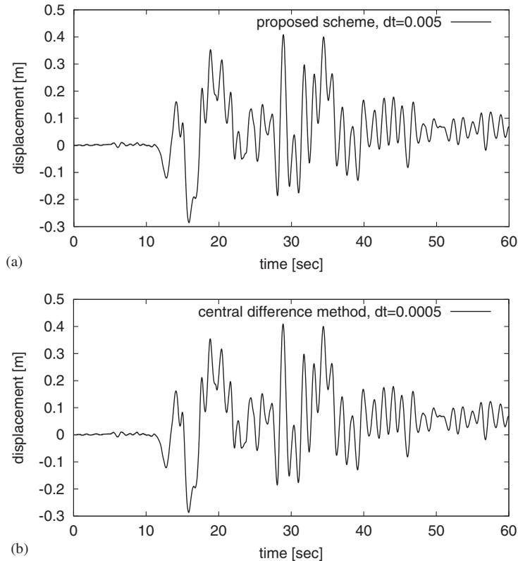
Figure 10. Comparison of the computation results by the NITI scheme and the conventional central difference method: (a) NITI scheme ( $\Delta t = 0.005$  sec); and (b) central difference method ( $\Delta t = 0.0005$  sec).
