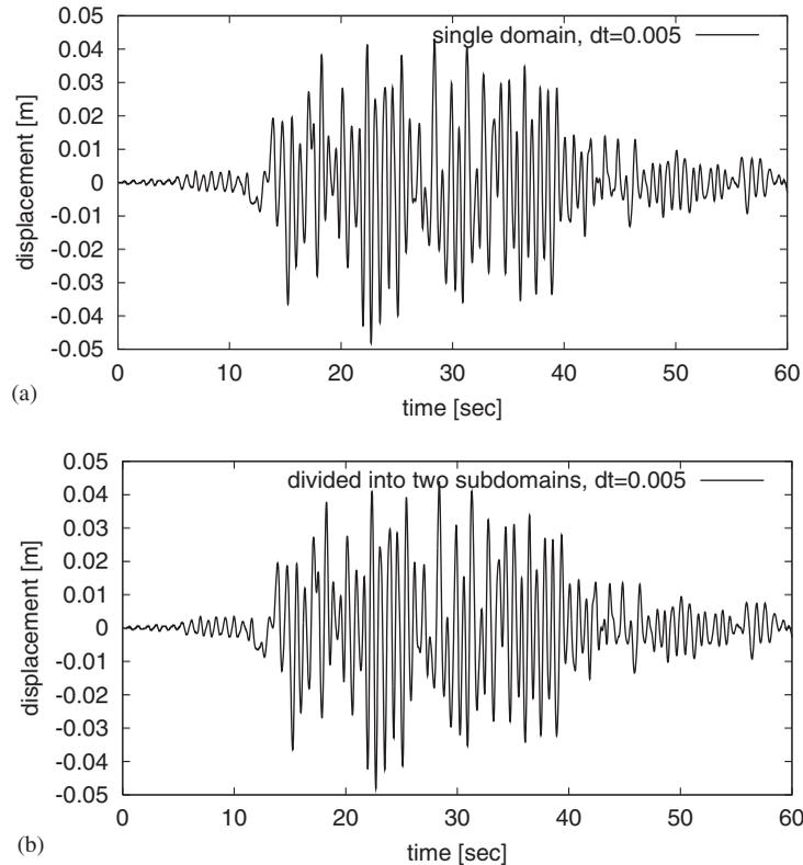
Figure 12. Comparison of the computation results by the FEM regarding the whole system as a single domain and that by the proposed scheme dividing the system into two subdomains ( $\Delta t = 0.005$  sec): (a) FEM with a single domain; and (b) FEM with two subdomains.
