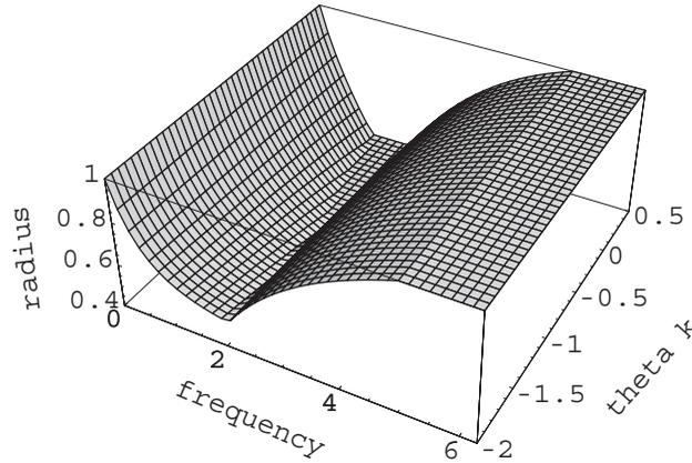
Figure 5. Relation of the radius, frequency  $\omega$  and  $\theta_k$  for the large damping factor  $h = 1.0$ ;  $\theta_c = 0.2$  is assumed.
