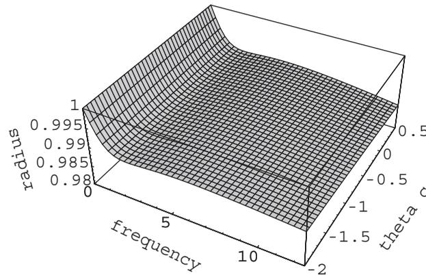
Figure 4. Distribution of the radius of the proposed scheme for various levels of velocity-dependent non-linearity.  $\theta_k = -0.1$  (stiffness decrease), and  $h = 0.01$  are assumed.
