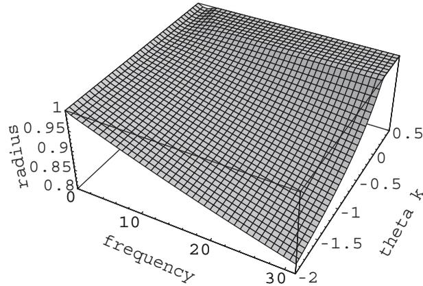
Figure 3. Distribution of the radius of the proposed scheme applied to the stiffness softening problem with velocity-dependent non-linearity.  $\theta_c = 0.8$  and  $h = 0.01$  are assumed.
