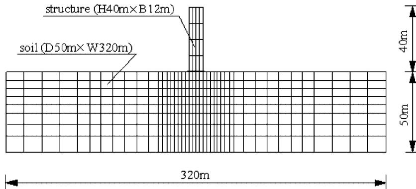
Figure 8. 2D soil–structure model.
