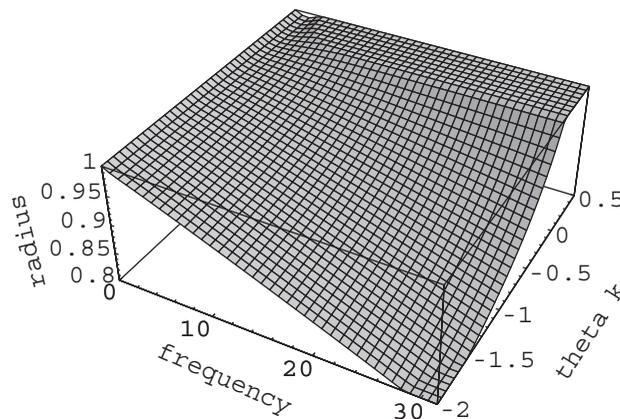
Figure 1. The radius for various frequencies  $\omega$  and  $\theta_k$  ( $\theta_c = 0$  and  $h = 0.01$ ).
