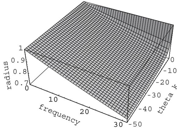
Figure 2. Distribution of the radius of the proposed scheme applied to the problem in which stiffness decreases to 1/50 of the initial value ( $\theta_c = 0$  and  $h = 0.01$ ).
