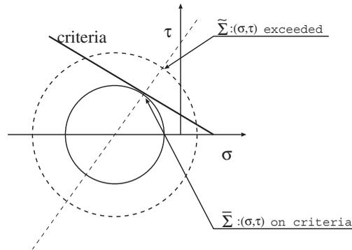
Figure 7. Stress used in the analysis of elasto-plastic material following Mohr–Coulomb’s fracture criteria.
