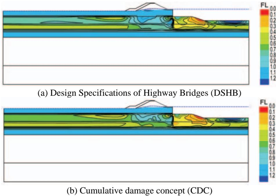
Figure 9. Distribution of the resistant factor against liquefaction  $F_L$ . (Subduction earthquake, 3K000 Left bank)
