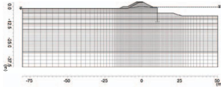
Prefecture Design Seismic Motion 2003). We computed the input earthquake motions at the engineering seismic base layer by 1-dimensional equivalent-linear earthquake response analysis code, DYNEQ (Yoshida and Suetomi 1996). Empirical equations reported by the Public Works Research Institute (Iwasaki et al. 1977, Iwasaki et al. 1980, Yokota and Tatsuoka 1982) are used for the dynamic deformation characteristics of soil in the analysis. The simulated input waves are shown in Fig. 6.
