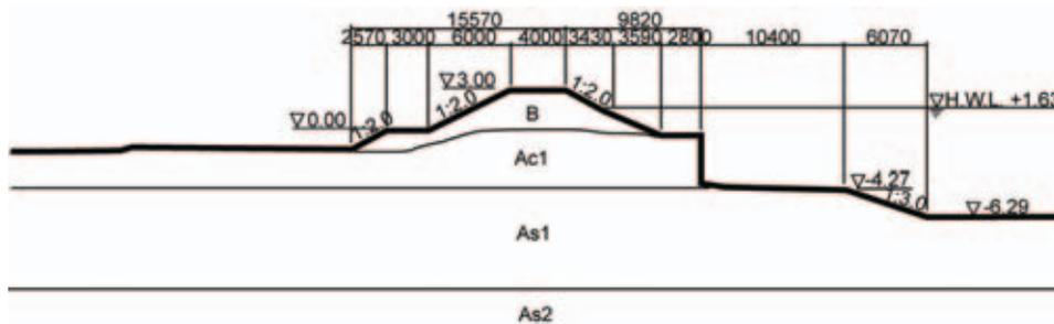
Figure 5. Outline of the river dike structure at the 3K000 Left bank.
