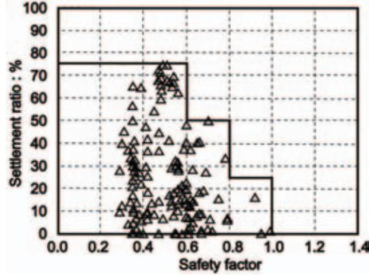
Figure 1. Relationships between the safety factor and the settlement ratio defined as settlement over height of dike (Japan Institute of Construction Engineering, 2002). The triangles are past damage and the solid line is the relationship used in evaluating the settlement from the safety factor.
