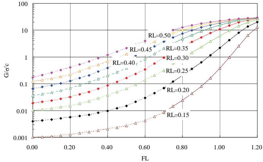
Figure 8. Relationship between the reduced shear rigidity ratio and the resistant factor against liquefaction (Yasuda et. al. 2005).
