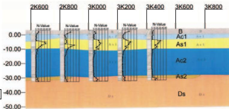
Figure 3. Soil profile along the left bank (River Works Office of Aichi Prefecture 2003)
