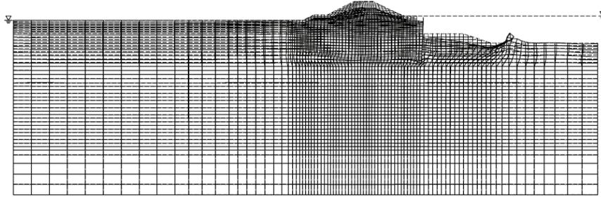
Figure 10. Deformation based on the liquefaction-induced flow analysis (Subduction earthquake, 3K000 Left bank).
