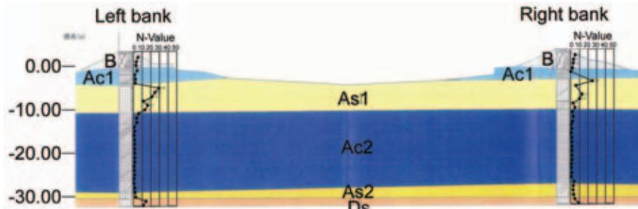
Figure 4. Soil profile at the 3K400 (River Works Office of Aichi Prefecture 2003)
